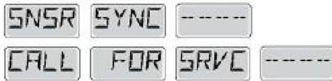
The temperature sensors ARE out of sync. The Sensor Balance is Poor fault has been established for at least 1 hour. Call for Service.
