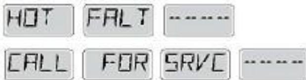
A pump appears to have been stuck on when the spa was last powered on. Water may be overheated.
