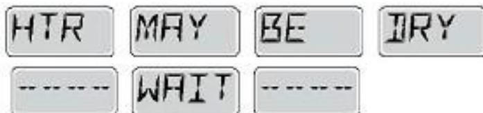
Possible dry heater or not enough water in the heater to start it. The spa is shut down for 15 minutes. Press any button to reset the heater startup.
